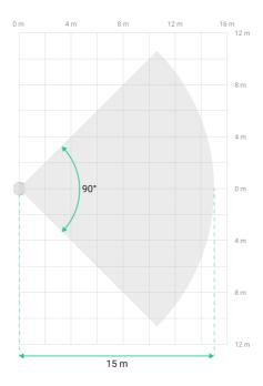
Horizontal characteristics of the motion detection area
