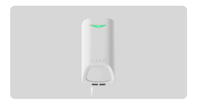
**Superior MotionProtect Plus G3 Fibra** is a wired motion detector. It detects movement at a distance of up to 15 meters. In addition to using the IR sensor, the detector applies an additional radio frequency scan with a K-band microwave sensor that filters out infrared interference. Also, it features an anti-masking system that detects attempts to block the detector's field of view. The device is designed for indoor use only and complies with EN 50131 (Grade 3) requirements.
