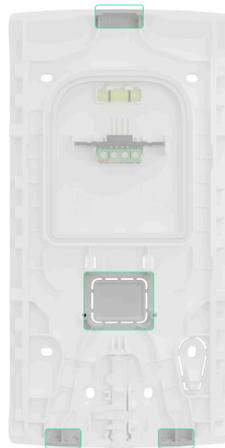
2. Route the cable of an unenergized power supply unit through the mounting panel.
