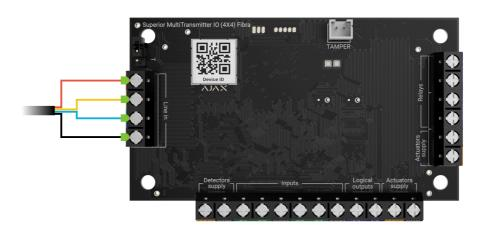
1. If Superior MultiTransmitter IO (4X4) Fibra is not the last device on the Fibra line, prepare a second cable in advance. Connect the wires to the Superior MultiTransmitter IO (4X4) Fibra terminals according to the figure below.
