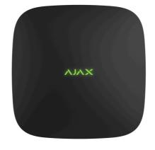
The ReX 2 Jeweller LED indicator may light up white, red, or green, depending on the status of the device and connection via Ethernet.
