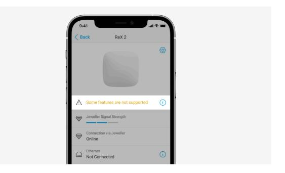
ReX 2 Jeweller can notify about malfunctions, if any. **Malfunctions** field is available in **Device States**. Clicking on (i) opens the list of all malfunctions. The field is displayed if a malfunction is detected.
