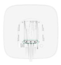
**4.** Slide ReX 2 Jeweller onto the mounting panel. After installation, check the tamper status in the Ajax app and then the quality of the panel fixation. You will receive a notification if an attempt is made to tear the range extender off the surface or remove it from the mounting panel.
