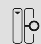
Additional input for connecting a thirdparty detector with the NC contact type
