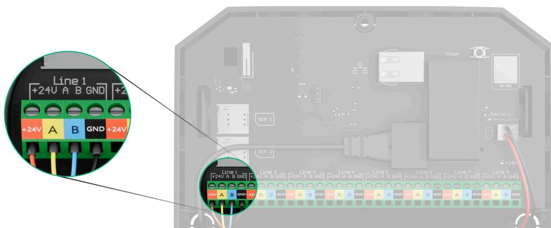
Hub Hybrid (2G) / (4G) has 8 Fibras lines. Numbers from 1 to 8 are indicated on the control panel board.
