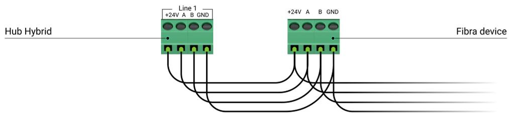
**+24V** – power supply terminal of 24 V $\overline{=}$ .
