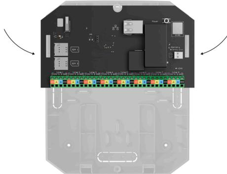
4. Connect the 12 V $\overline{=}$  backup battery. Do not connect third-party power supplies. This could result in a failure of the control panel.
