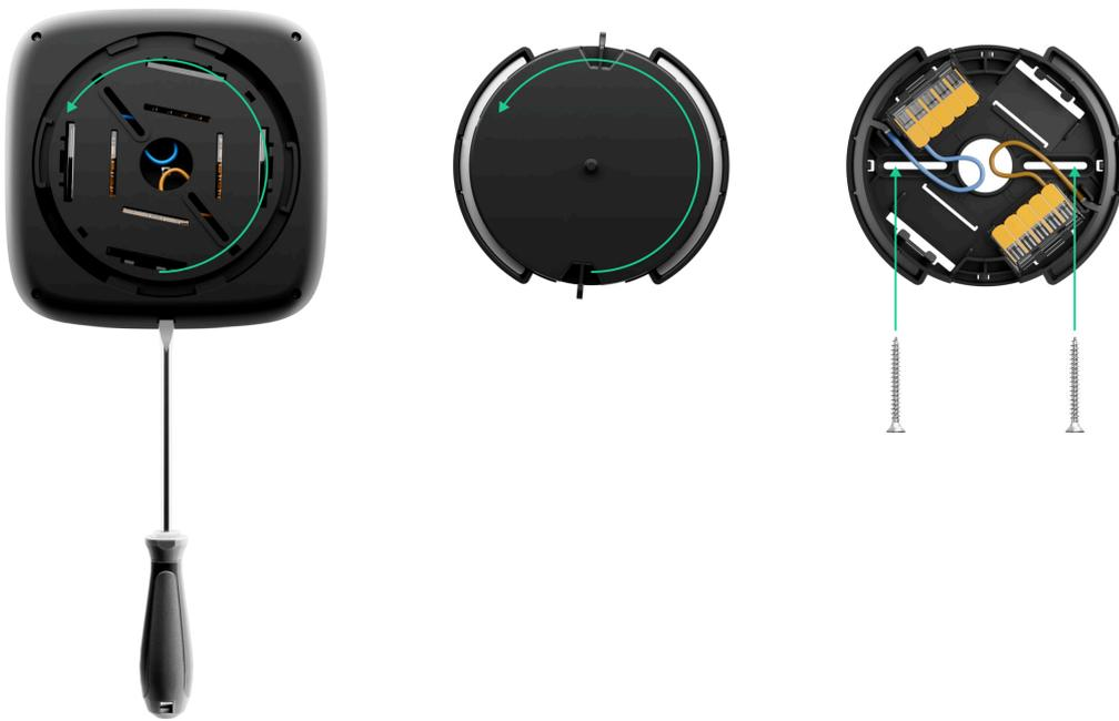
6. Power off the cable that you will connect to the detector. Route the external power supply cable through the hole in the attachment panel.
