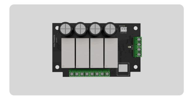
**Superior MultiRelay Fibra** is a module to control electrical appliances' power supply remotely. The device has four relays with electrically isolated dry contacts. The relays can control the power supply of electrical appliances connected to the circuit. To change the states of the relays, use the **Ajax apps**, create **automation scenarios**, or press **Button**.
