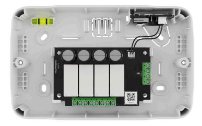
We recommend installing MultiRelay into Case. The casing is sold separately and available in multiple versions. Installing a single module, several modules, or several other devices into Case is possible. Use **Case configurator** to get the most optimal placement of your Fibra devices in the casing.
