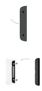
**9.** Tighten the holding screw on the bottom of the detector's and magnet's enclosure. The screw is needed for more reliable fastening and protection of the detector and the magnet from quick dismantling.
