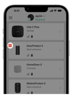
When a malfunction is detected, the Ajax app displays a malfunction counter on the device icon. All malfunctions are shown in the detector states. Fields with malfunctions will be highlighted in red.
