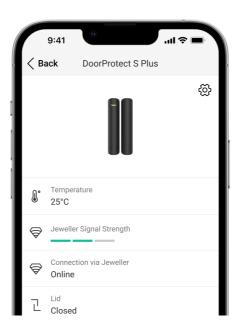
The states include information about the device and its operating parameters. The states of **DoorProtect S Plus** can be found in Ajax apps:
