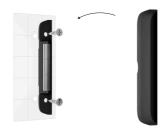
**9.** Tighten the holding screw on the bottom of the detector's and magnet's enclosure. The screw is needed for more reliable fastening and protection of the detector and the magnet from quick dismantling.
