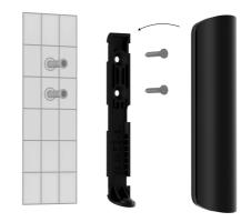
**3. To mount a small magnet**: disassemble its enclosure by prying up the back with a flat object. Use a slotted screwdriver for this. Fix the part with magnets on the surface; use the bundled screws for this. Then install the front panel in its place.
