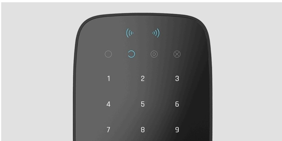
KeyPad S Plus can be used in low-light conditions as it has a backlight. Pressing the buttons is accompanied by a sound signal. The backlight brightness and keypad volume are adjustable in the settings. If the keypad is not touched for 4 seconds, KeyPad S Plus reduces the backlight brightness. After 8 seconds of inactivity, it enters power-saving mode and turns off the display.
