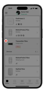
When a Superior Transmitter Fibra malfunction is detected, the Ajax app displays a malfunction counter on the device icon. All malfunctions are indicated in the module states. Fields with malfunctions will be highlighted in red.
