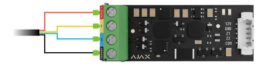
If Superior Transmitter Fibra is not the last device on the Fibra line, prepare a second cable in advance. Connect the wires to the Superior Transmitter Fibra terminals according to the figure below.
