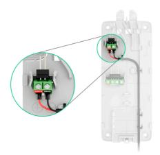
**4.** Once the keypad is <u>installed</u> and added to the hub, check the status of the backup batteries and external power in the Ajax app, as well as the overall operation of the device.
