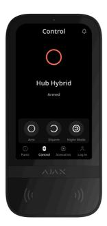
Superior KeyPad TouchScreen Fibra can arm and disarm the entire object or specific groups, and activate **Night mode**. Use the **Control** • tab to change the security mode. Users can control the security using Superior KeyPad TouchScreen Fibra through:
