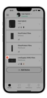
When a LineSupply malfunction is detected, the Ajax app displays a malfunction counter on the device icon. All malfunctions are indicated in the module states. Fields with malfunctions will be highlighted in red.
