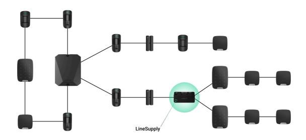
While Ajax systems support **Beam** and **Ring** topologies, avoid connecting the module's Fibra output lines in a **Ring** topology.
